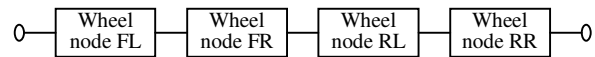
Figure 8. RBD for the wheel node subsystem with full functionality mode and FS nodes
