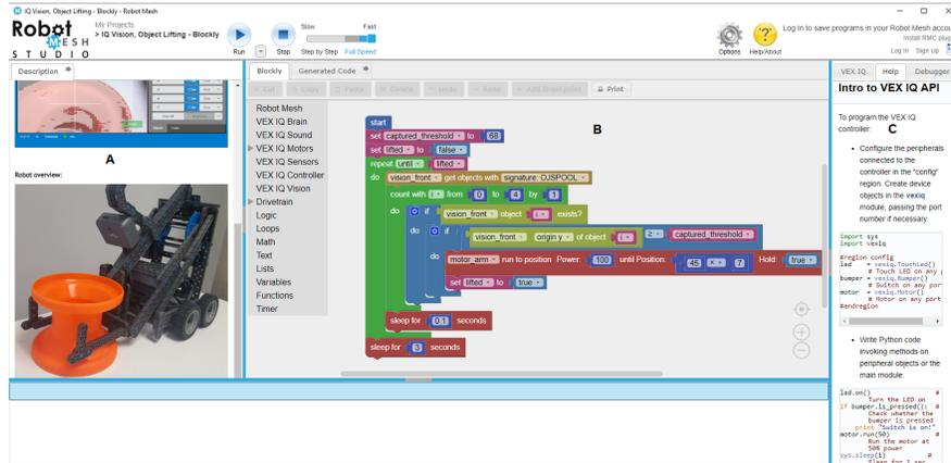
**Fig. 1** Screenshot of the Robot Mesh Studio IDE [78] with three panes. Pane A provides an rich-text description of the mission, Pane B the actual mission expressed in a DSL with Blockly syntax, and Pane C shows help text or alternatively the debugger or an overview on the current robot configuration.
