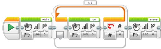
**Fig. 6** Specifying a loop in LEGO Mindstorms EV3.
