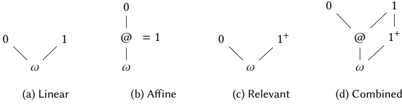
Fig. 2. Hasse diagrams for various substructural type system lattices. The modality @ corresponds to 0 or 1 uses, 1^+ corresponds to 1 use or more, \omega corresponds to any number of uses.
