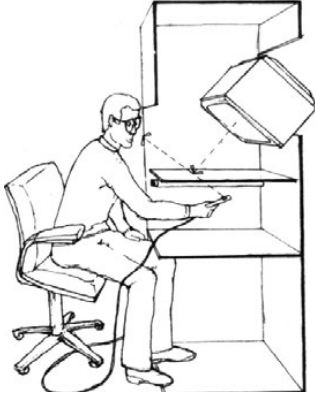
Figure 8. A sketch from Schmandt of his Workbench. A cutaway view of the work station, showing the view through the half silvered mirror of the video monitor and the user's hand [27].
