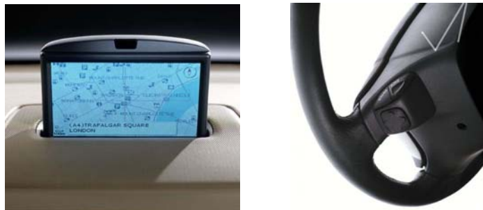
Figure 4: Shows the navigation display (left), the Back - and Enter -buttons and the four-way switch on the underside of the steering wheel (right).
