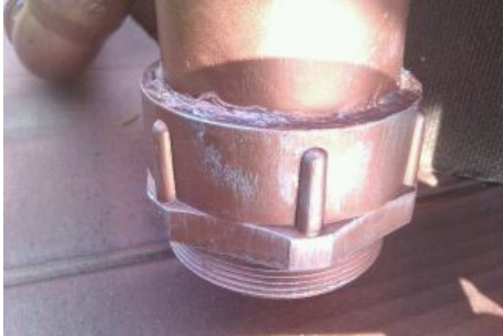
Figure 3: Shows paint detail and the fake welding.
