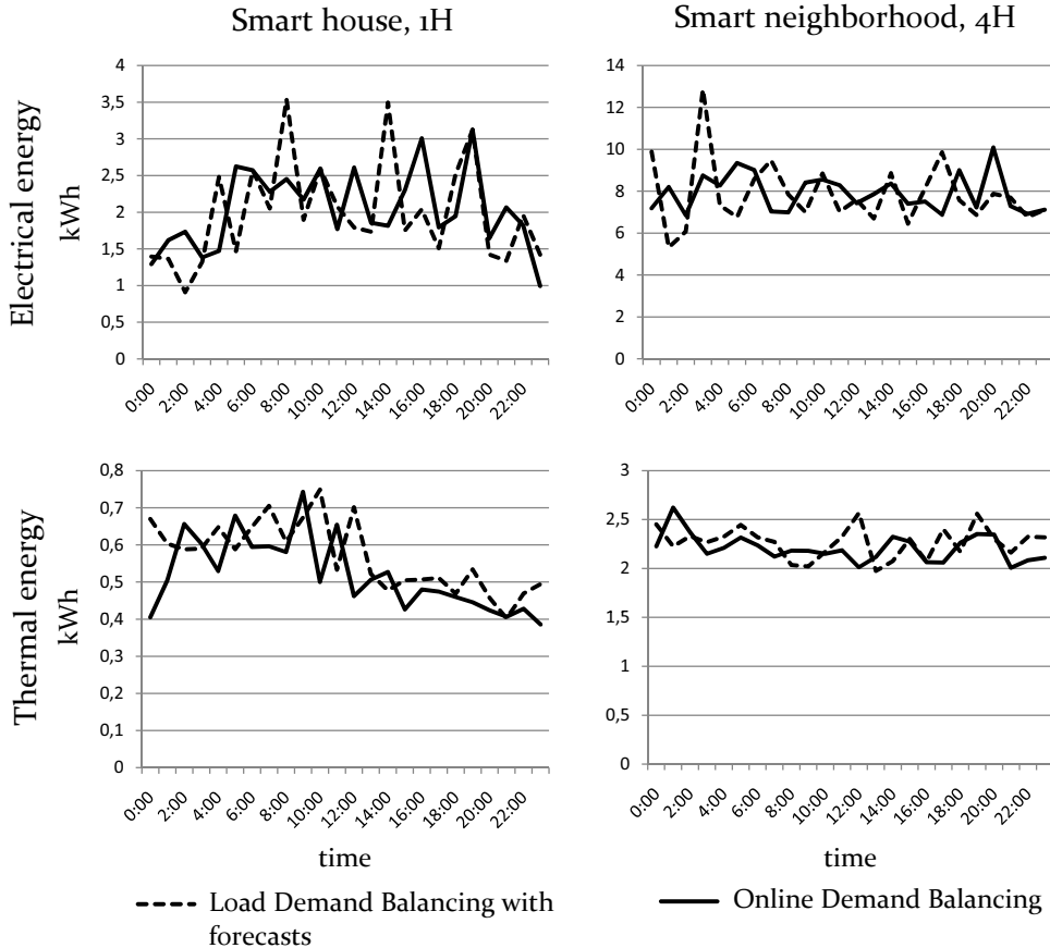
Figure 8: Comparison of load demand curves for the Smart house/neighborhood scenario for one and four household(s)
