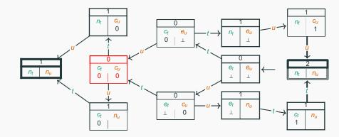
Mutual exclusion in writing to counter:  $\Box \neg (ct \land cu)$ , with *nt* denoting that *t* is not in its critical section, and *nu* denoting that *u* is not in its critical section
