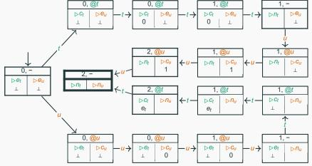
Mutual exclusion in writing to counter:  $\Box \neg (ct \land cu)$ , with *nt* denoting that *t* is not in its critical section, and *nu* denoting that *u* is not in its critical section
