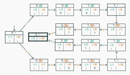
Tracking every statement can lead to large state diagrams We can simplify a diagram by skipping lines irrelevant to concurrent behavior
