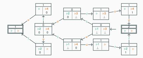
The state/transition diagram of the concurrent counter example using locks should contain no (states representing) race conditions:
