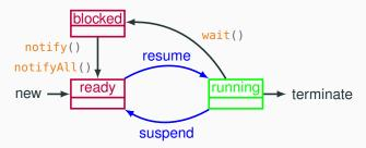
Waiting and notifying only affects the threads that are locked on the same shared object (using **synchronized** blocks or methods).
