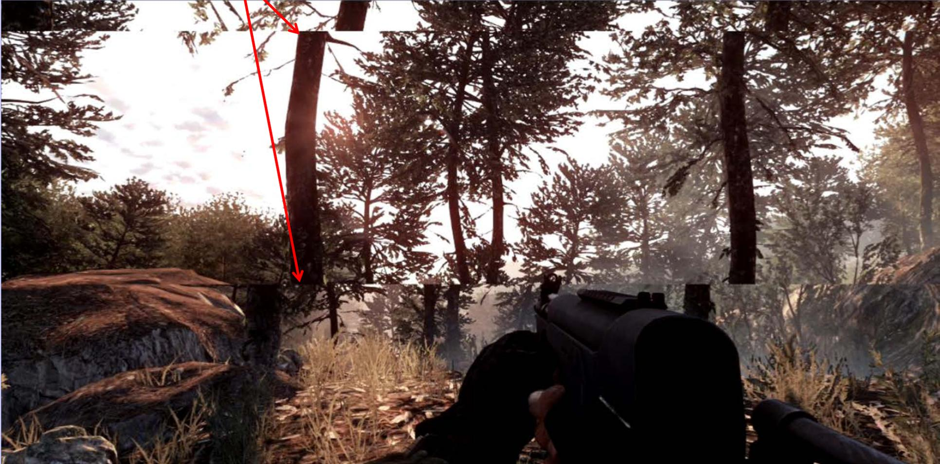
Screen tearing is solved by using V-Sync.
