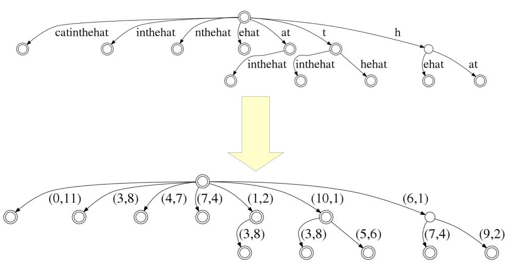
(need to also remember that the input string is catinthehat) This takes O(n) memory! (Recall that a radix tree containing n values has at most 2n nodes)
