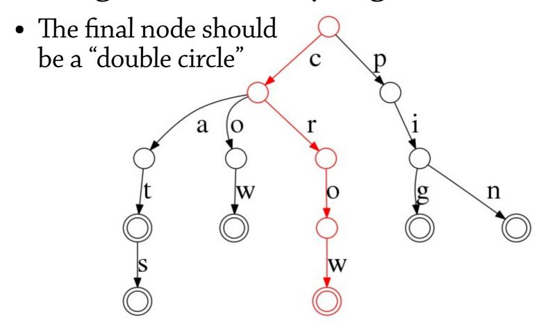
Inserting "pi" creates no new nodes, but we mark the final node as a "double circle"
