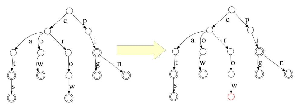
If the node is a leaf, we should remove it. We go up the tree removing any single-circled leaves, which restores the invariant:
