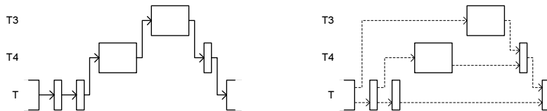
(b) T allocates T3 and T4. T evaluates T4 which in turn requires T3 to be evaluated.
