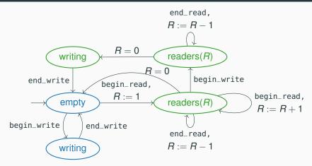
By inspecting the diagram we can understand that it guarantees fairness provided outgoing transitions from the same state have the same priority (they are served in arrival order). The solution in Erlang implements the behavior of this diagram, using two server functions empty\_board and readers\_board which call each other.
