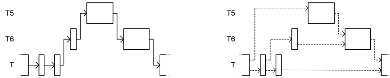
(c) T allocates T5 and T6. T evaluates T6 which immediately requires T5 to be evaluated.
