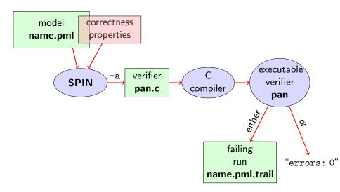
Given Promela model M, and correctness properties  $C_1, \ldots, C_n$ .
