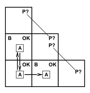
Breeze in (1,2) and (2,1)  $\Rightarrow$  no safe actions Assuming pits uniformly distributed, (2,2) has pit w/ prob 0.86, vs. 0.31
