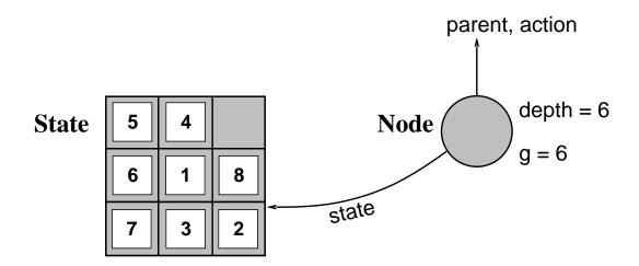
The  $\rm Expand$  function creates new nodes, filling in the various fields and using the  $\rm SuccessorFn$  of the problem to create the corresponding states.
