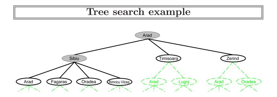
Note: Arad is one of the expanded nodes! This corresponds to going to Sibiu and then returning to Arad. Implementation: states vs. nodes
