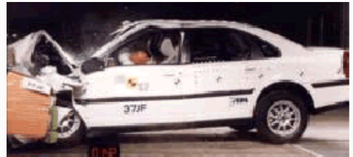
Offset crash test at 64km/h
