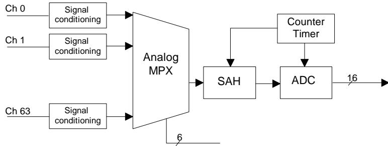
The *Done* bit is reset. The sampled value is converted to a binary value and placed in a 16 bit data register located at FFFFFFF02. The *Done* bit is now set. If the *Interrupt Enable/Disable* is set an interrupt is generated. Write an ADA package AD\_Converter with a single procedure, using *Interrupt Enable*:
