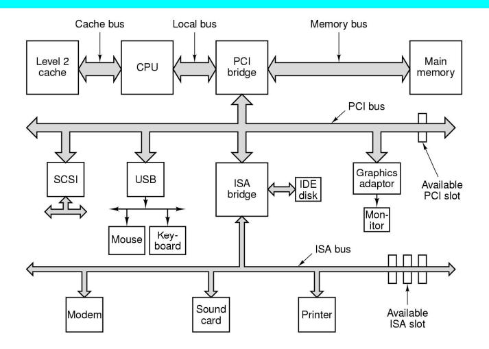
Structure of a large Pentium system (Fig, 24 from Modern OS, A. Tanenbaum)
