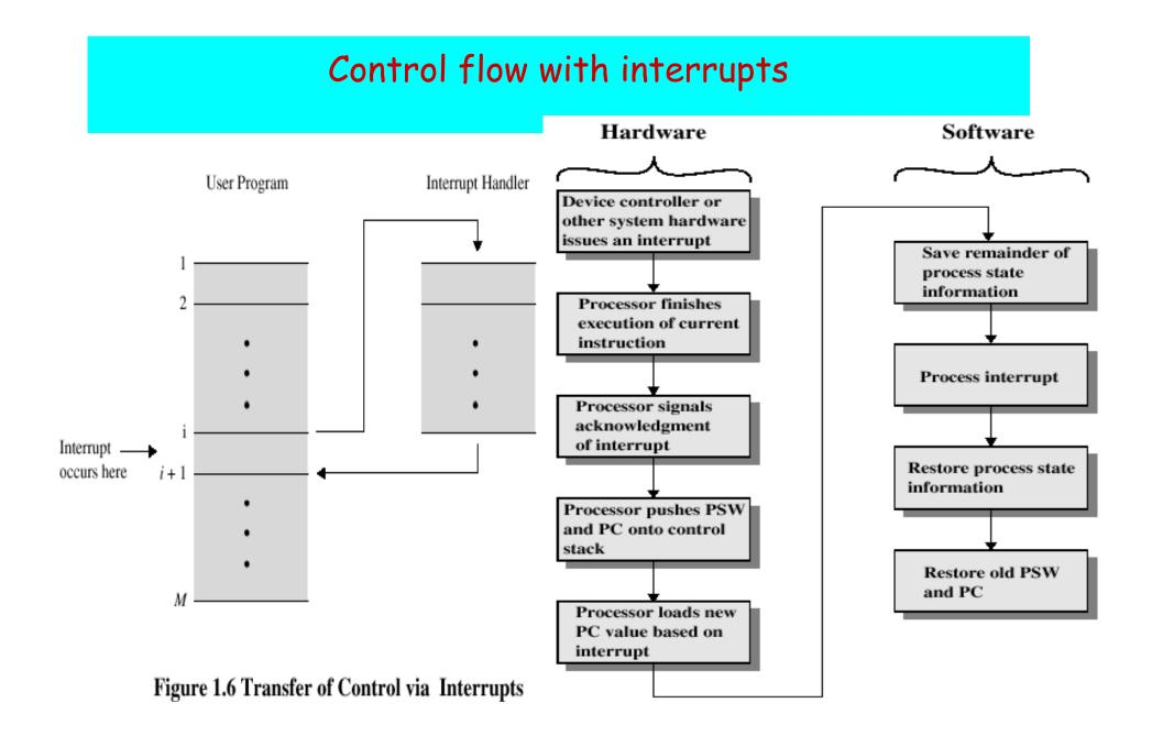
Figure 1.10 Simple Interrupt Processing
