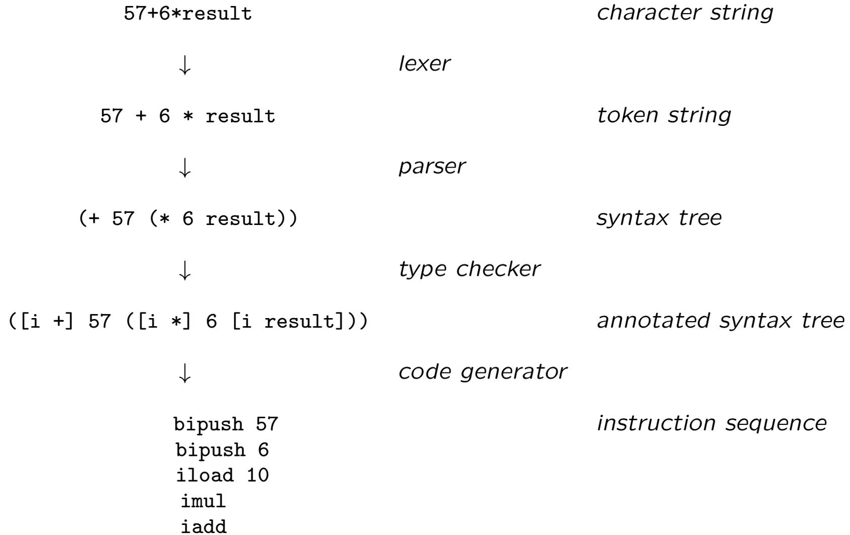
**Compilation phases from Java source code to JVM assembly code**
