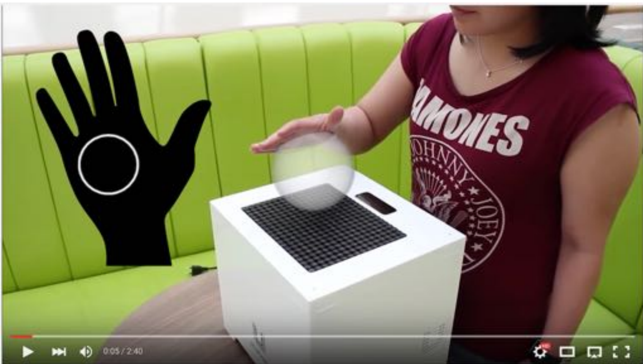
Rendering Volumetric Haptic Shapes in Mid-Air using Ultrasound
