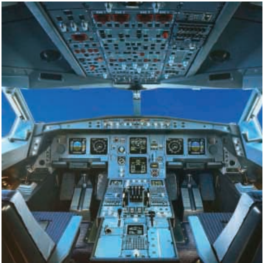
The controls of a SAS Airbus 340 feed in to a "fly-by-wire" computer system, which is responsible for mechanically controlling the aircraft. A missed deadline or logical error could have disastrous consequences. Photo: SAS
