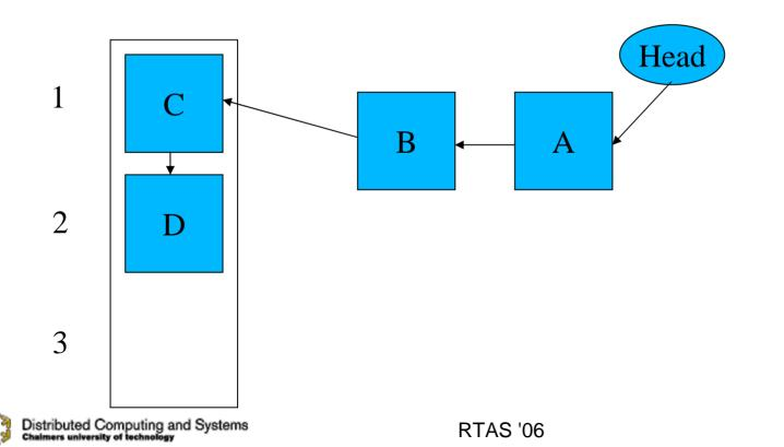
• We go through the tail array looking for the node that doesn't point to another node
