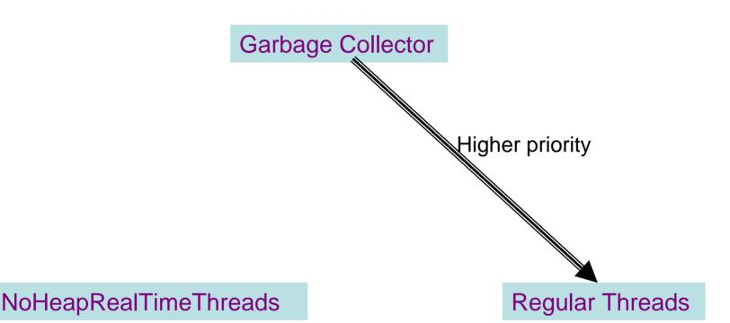
Regular java threads must wait until the collector reaches a preemption-safe point.
