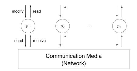
Figure 2.3: Interaction with a distributed shared memory. The application can communicate with familiar operations as read and modify with processes which implement the required memory consistency.
