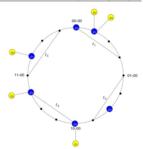
Figure 6.1: Forwarders and children in a role-based DHT allowing a maximum of four topics and four processes.
