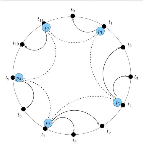
Figure 5.4: Illustration on how processes maintain and coordinate vector clock entries. An arrow from process  $p_i$  to a vector element indicates that  $p_i$  is the respective coordinator.
